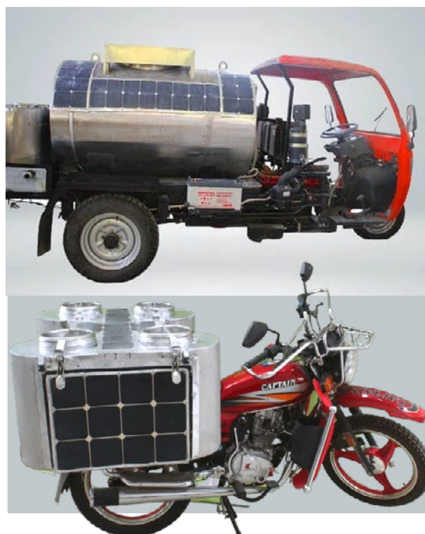
Solar cooling milk chillers
