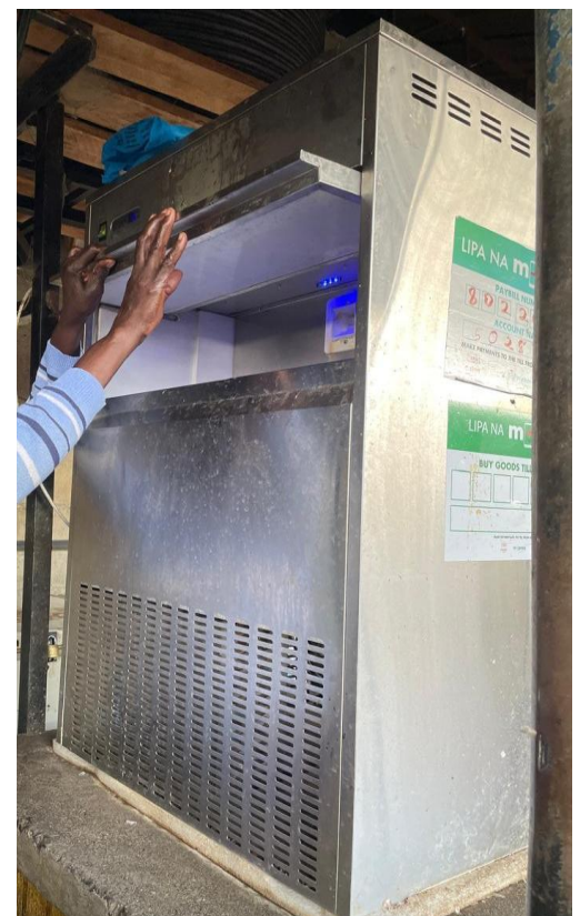
Figure 2: An Ice Flake Machine installed at the Ukulima Market
