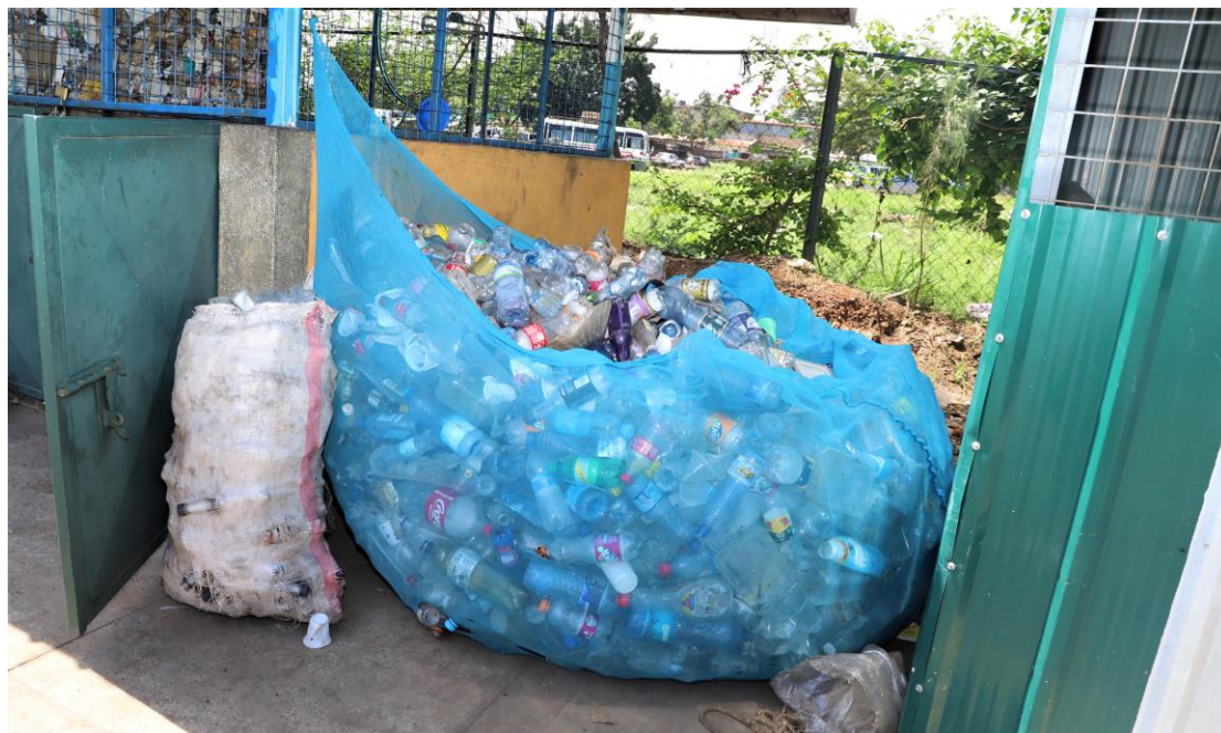
Plastic waste sorting zone: Plastics awaiting cleaning, sorting by type, and shredding
